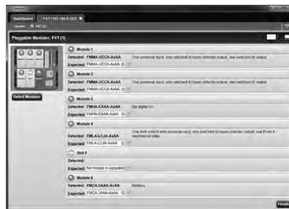
Pluggable modules view simplifies configuration by showing hardware present.
