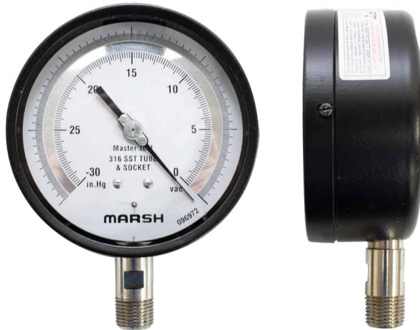
The Marsh Instruments Test Gauge is designed with a black painted steel housing and 316 stainless steel tube and socket to meet the demanding service needs of various test gauge applications. Accuracy is 0.5% of full span. A highly polished integral mirror is positioned between the two graduation arcs on the dial face. The knife-edge pointer is reflective so that, when the pointer and its reflection are in alignment, parallax is virtually eliminated and a true dial reading is assured.
